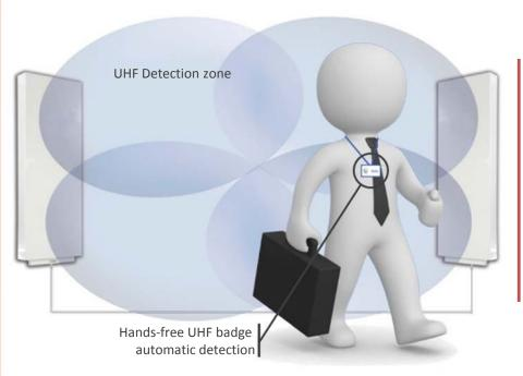
The UHF hands-free reader can identify a moving person in a 2 or 4 meter wide corridor by reading a UHF tag. Single or dual-antenna configurations are possible, depending on the area to be covered. Can be installed indoors or outdoors. Optional passage sensor (counter, direction and detection).
