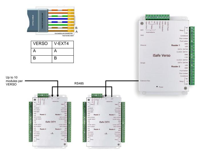
You can also use the A and B terminals on the V-EXT4 modules to connect an RS485 bus.
