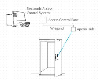
Local wireless communication eliminates the cost and inconvenience of wiring in and around the door, without the hassle of complex site surveys.
