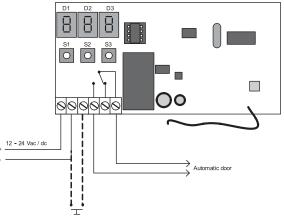
It is necessary to use a separate Power Supply for the Electric Lock
