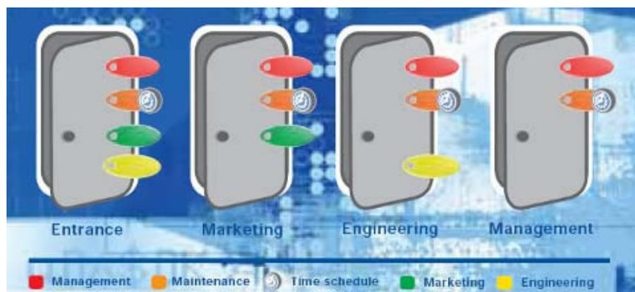
RFID enables contactless identification of transponders within tags/cards. MIFARE supports ISO14443/A, 13.56 MHz. The technology is embodied in both tags and readers, with a typical read/write distance of 2 cm. Unlike with other RFID solutions, the short range assures high protection of data transmissions between tag and reader.
